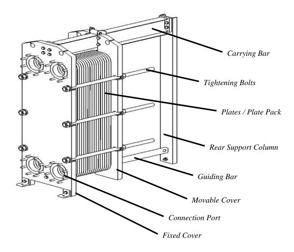
The frame is made up of thick steel pressure retaining parts, the *fixed cover* and the *movable cover*, that when pulled together with the *tightening bolts* form the pressure retaining structure for the *plates / plate pack*.
