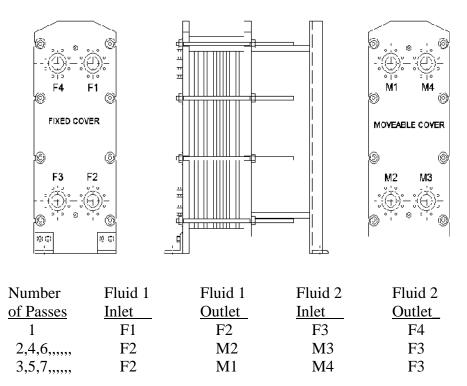
An assembled unit must always have the plate chevron pattern rotated 180 degrees from plate to plate.
