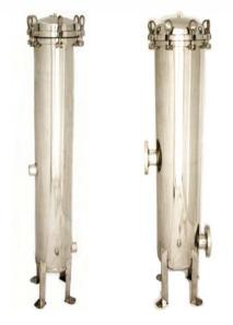
The WesFlo<sup>®</sup> 4NCF non-code, multi-cartridge filter vessels provide an economically efficient means of filtration for a wide variety of liquid applications. With a lightweight, externally polished stainless steel design, these vessels also include a swing bolt closure and internal positive pressure cartridge alignment and sealing plates.
